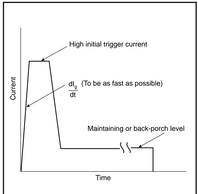
**Fig.2 Output load line for gate drive**
