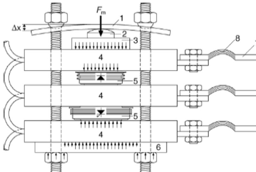
Figure 13 Example of a stack, illustrating the basic rules for correct clamping of Press-Pak high power Semiconductors:
