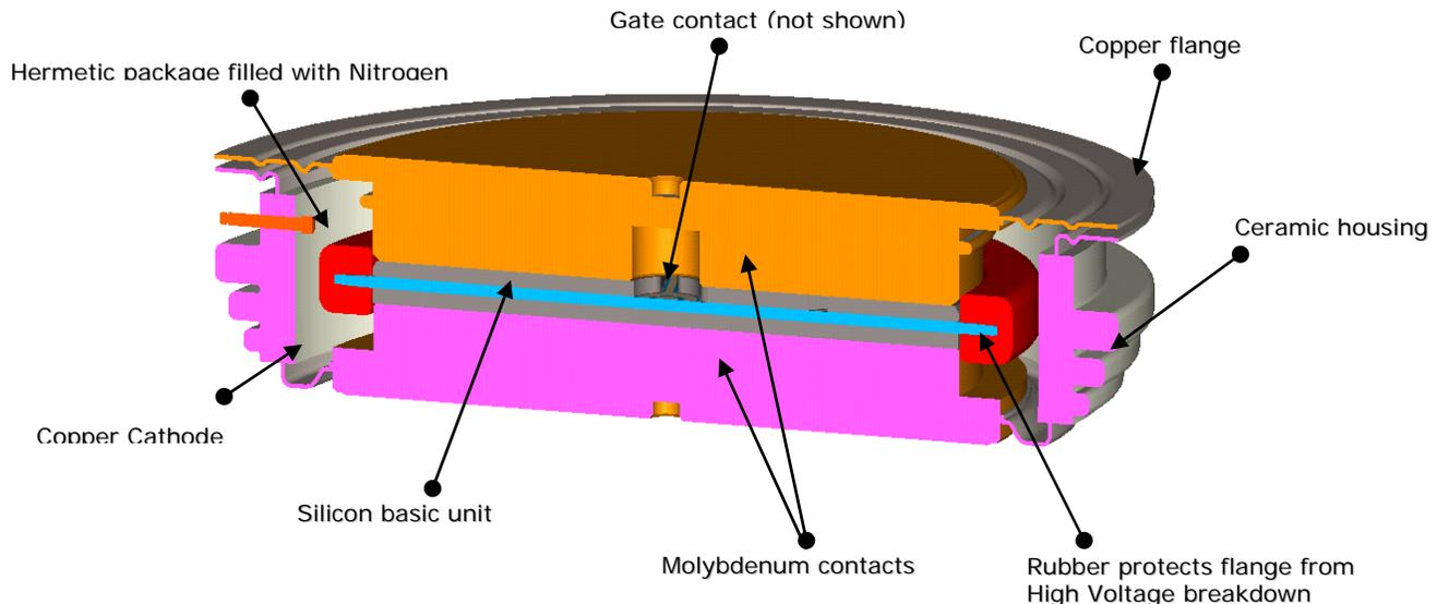
Figure 1. Internal Construction of typical Free-Floating Press-Pak Semiconductor
