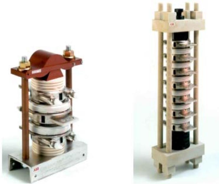
Figure 8-9. Two rods are enough for shorter stacks, but for longer stacks 4 rods are recommended.
