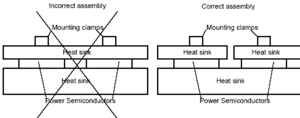
**Figure 10 Devices should be individually clamped.**
