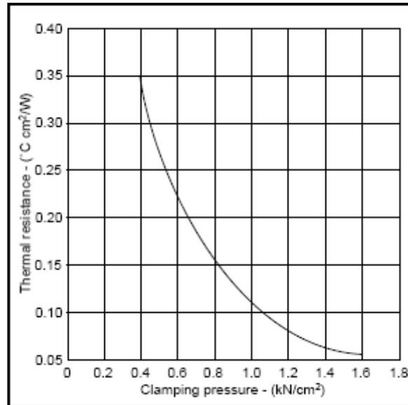
**Fig.2 Additional thermal resistance for dry interfaces of a Free Floating Semiconductor Press-Pak**
