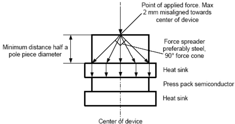
Figure 7 Recommended application of the mounting force.
