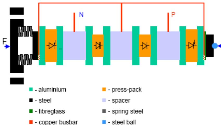
Figure 12 Poorly designed stack with ineffectual load spreaders and dissimilar device diameters.
