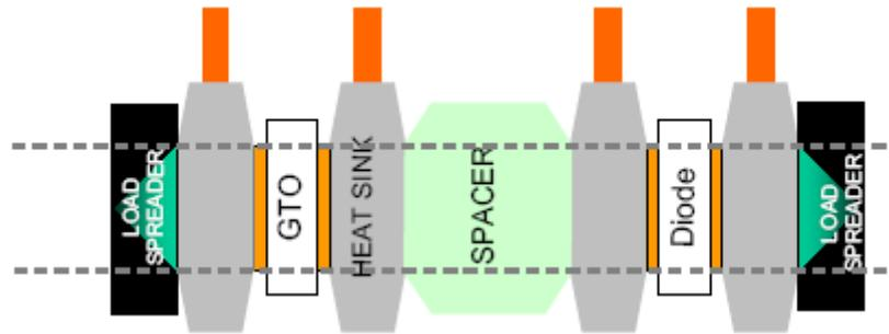
Figure 11 Well designed stack with effective load spreaders and similar device diameters.
