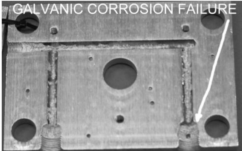
**Figure 7. Photo of an aluminum SCR cooling block showing Galvanic Failure**
