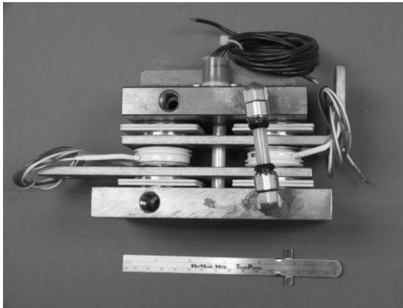
**Figure 5. Photo of indirectly cooled SCR contactor – double side cooled - copper**
