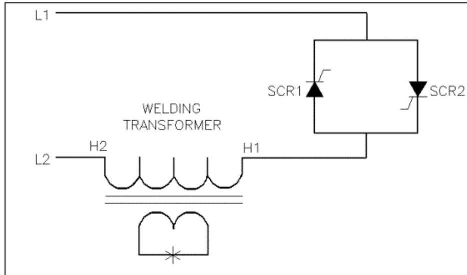
**Figure 1. Diagram of SCR Contactor and Welding Transformer**
