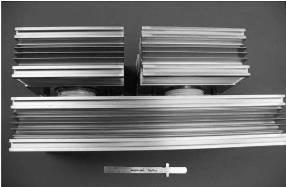
**Figure 3. Photo of Air Cooled SCR Contactor**
