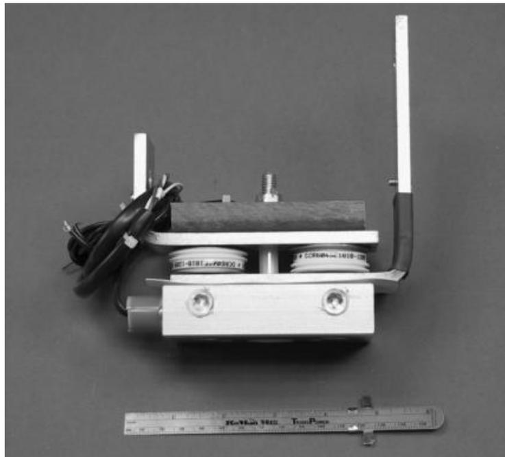
**Figure 6. Photo of indirectly cooled SCR – single side cooled - aluminum**
