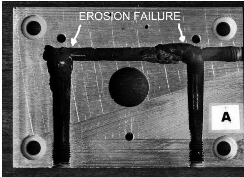
**Figure 9. Photo of an aluminum SCR cooling block showing Corrosion Assisted Erosion**
