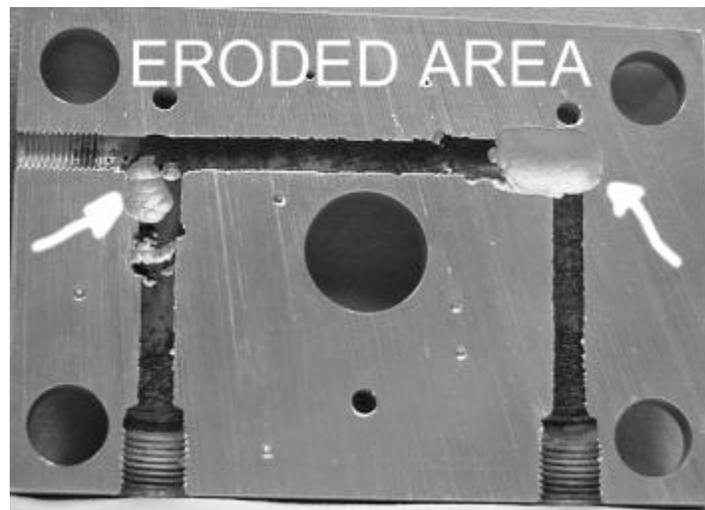
**Figure 8. Photo of an aluminum SCR cooling block showing Erosion**
