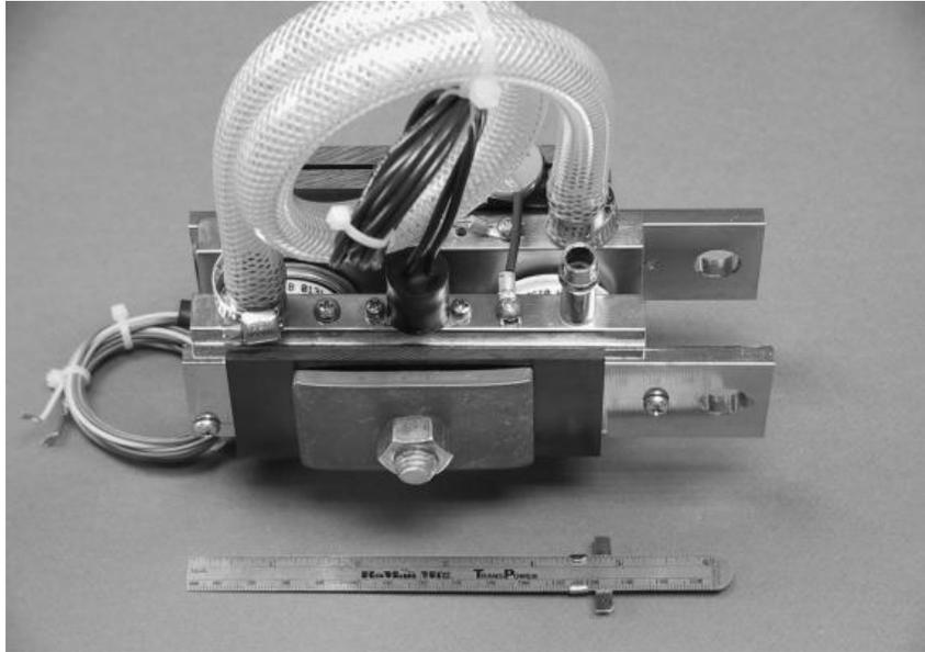
**Figure 4. Photo of Direct Water Cooled Contactor – double side cooled**
